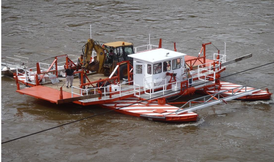
Figure 2: Picture of a reaction ferry in action. (British Columbia Provincial Government, n.d.)
