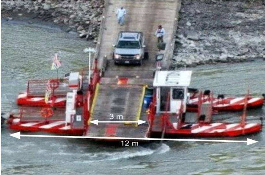
Figure 9: Picture of a truck boarding the Lytton Reaction Ferry (Mike, 2013) Dimensions estimated by Tan (2022).
