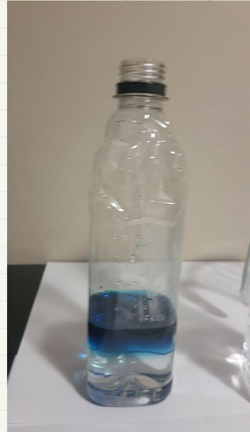
The respirometer just as we added the bromothymol. The bromothymol is above the water.
