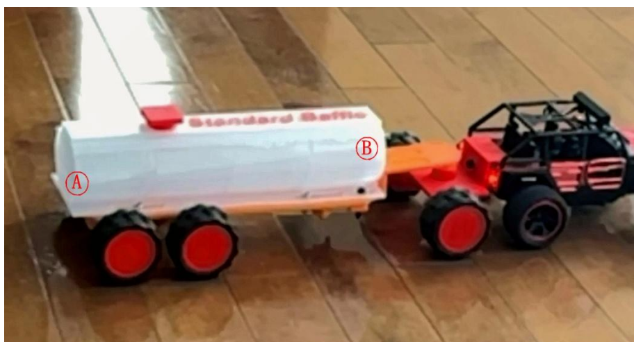
Figure 9: Sloshing Level of Standard Baffle
