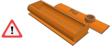
My second design failed as the lid did sit flush on the top of the base part of the tanker, but it had nowhere to grab on to, eventually falling into the base. I learned that I needed to create a groove to allow the lid to stay securely.
