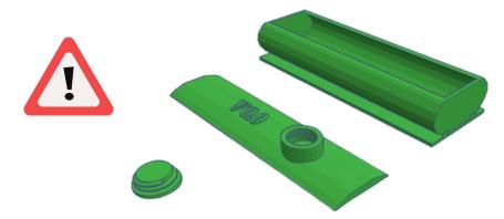
My first design was a very tiny closed one piece tank, however, due to a 3D printer's limitation, it is unable to print overhangs (a part of the model that extends outward without support underneath).
