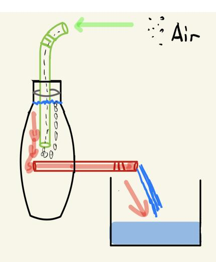
The green straw has a vacuum pump attached to it and it is sucking in the air.
