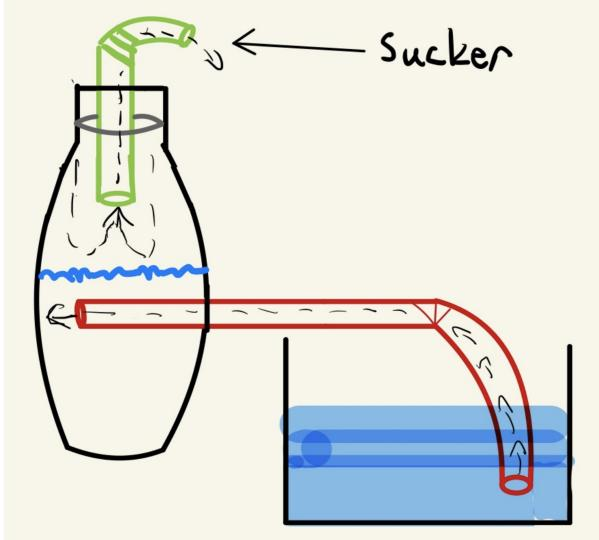
The water level is below the red straw's lowest point inside the bottle of water and air is getting pumped in.
