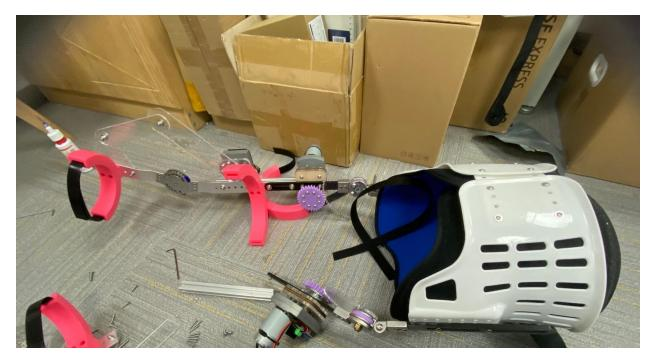
Started assembling cables and pressure sensors and connecting them to the gears and continued with bonding the wires.
