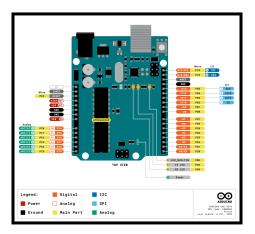
be used for both digital input and digital output. PWM is a technique used to encode a message into a pulsing signal. They are composed of 2 components: frequency and duty cycle. PWM frequency dictates how long it takes to complete a single cycle and how quickly it fluctuates from high to low. The cycle determines how long a signal stays high out of the total period. Finally, Serial, Serial communication is used to receive and transmit data between the Arduino board and another serial device.
