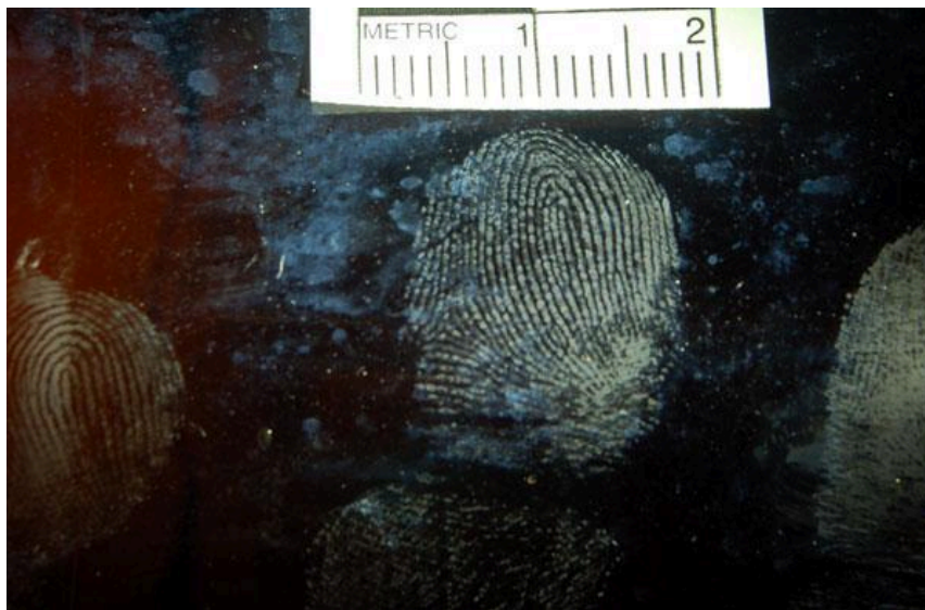
Super glue fumes cling to latent fingerprints on the neck of a glass bottle.
