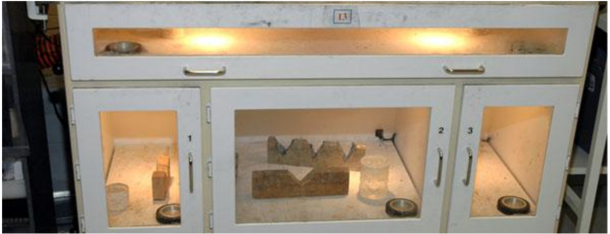
A specially designed chamber for exposing latent prints to super glue fumes.
