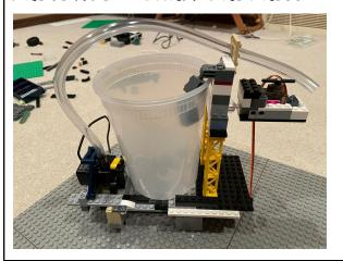
On the first day we started to build the structure of the robot out of Lego,and secured the water pump and the servo motor. I also attached the tube to the water pump that went through a frame structured Lego piece to center the tube better. We positioned the water tank in the middle with a hole in its side connecting to the other tube of the water pump.
