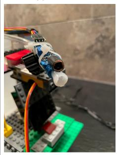
Here is the nozzle with a spray nozzle at the end of the pipe. On the top the flame sensor is mounted and attached by zip ties the end of the fire sensor has some tape so it helps the robot pinpoint it more precisely making it easier to extinguish the flame.
